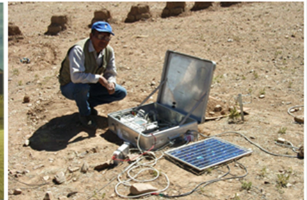
Fig. 4.1: Above left: Fundamental layout in the field (DL: data logger). The probes are in a cross layout. Above right: Connection of the telluric probes at the input of an operational amplifier. Below left: Layout of telluric cables. Below right: View on data logger, electronics for controlling the fluxgate magnetometer, external GPS for time synchronization and solar
